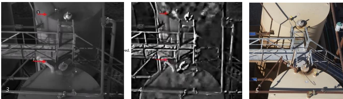
Image 3, 4, & 5: Left: A still image from drone OGI video in normal mode. Middle: A still image from drone OGI video in enhanced mode. Right: Image from normal digital camera.
